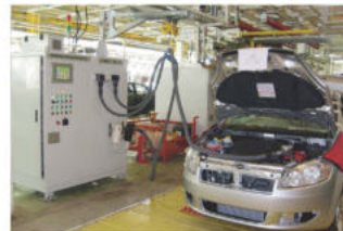
Washer Fluid Filling Equipment
